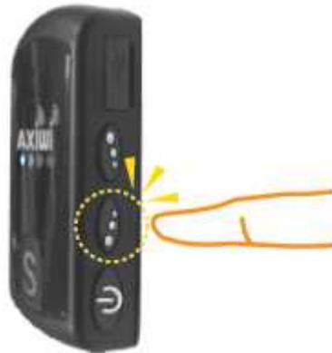
The cut-off function is to allow the master mode unit to cut off the permission to speak mode from ALL slave units. When active none of the slave units on the current channel can use the permission to speak function.
