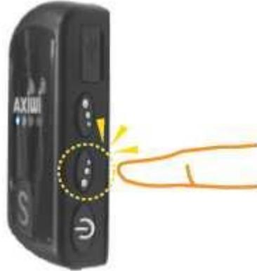
The cut-off function is to allow the master mode unit to cut off the permission to speak mode from ALL follower units. When active none of the follower units on the current channel can use the permission to speak function.
