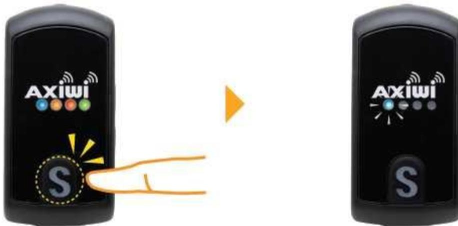
\* This function is to allow a follower mode device to cancel its permission to speak by the user himself/herself. When in normal "listening mode", only one LED for the specific channel on the unit will be blinking, instead of four lit LEDs.
